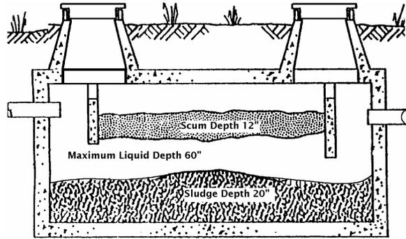
5. Add the scum and sludge depth measurements. If they total more than half of the total depth of the tank, then it is time to clean the tank.
